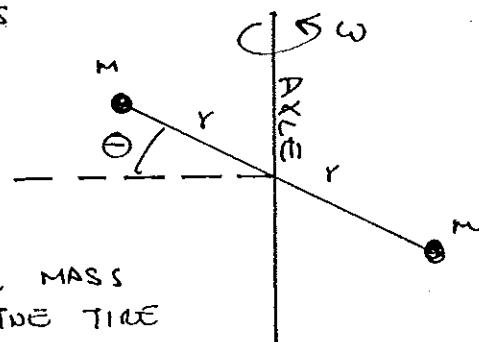
IN THIS PROBLEM IGNORE ALL OTHER MASS OF THE TIRE EXCEPT THE  $2m$ . SUPPOSE THE TIRE IS NOT ROLLING, BUT IS IN A SPECIAL SET-UP WITH THE AXLE VERTICAL & THE C.M. FIXED - THE "BALANCING" DEVICE.
