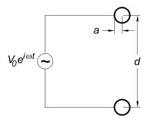
The internal resistance of the source is zero, but a reactance exists due to the capacitor formed by the two terminals, which are taken to be conducting spheres of radii a, separated by a distance  $d \ll \lambda$ , where  $\lambda = 2\pi c/\omega$  and c is the speed of light.
