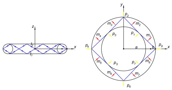
Each of these loops has a magnetic moment  $\mathbf{m}_j$  that is perpendicular to the plane of each loop, and which lies in the x-y plane, as shown on the right part of the figure.
