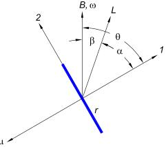
If the thin disc has mass m and radius r, then its inertia tensor has diagonal elements  $(I_{11}, I_{22}, I_{33}) = mr^2(2, 1, 1)/4$ . The initial angular velocity  $\boldsymbol{\omega} = \omega(\cos\theta, \sin\theta, 0)$  is parallel to **B**, at angle  $\theta$  to the  $\hat{1}$ -axis. The "mechanical" angular momentum of the precessing disc is,
