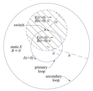
A conducting loop of radius a (the primary loop) contains a battery of potential difference V, and a switch that is initially open. Initially there is no electrical current, and no magnetic field **B**, anywhere, although a static electric field **E** due to the battery exists everywhere.
