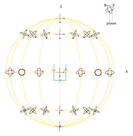
Figure 2: The elliptical polarization of the fields (12)-(13) of the U-shaped antenna in the limit of small h. From [7].
