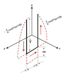
Figure 1: The U-shaped antenna whose radiation pattern is isotropic in the limit that  $h \to 0$ , for which the intensity also goes to zero. The dashed lines indicate the spatial dependence of the current. From [5].
