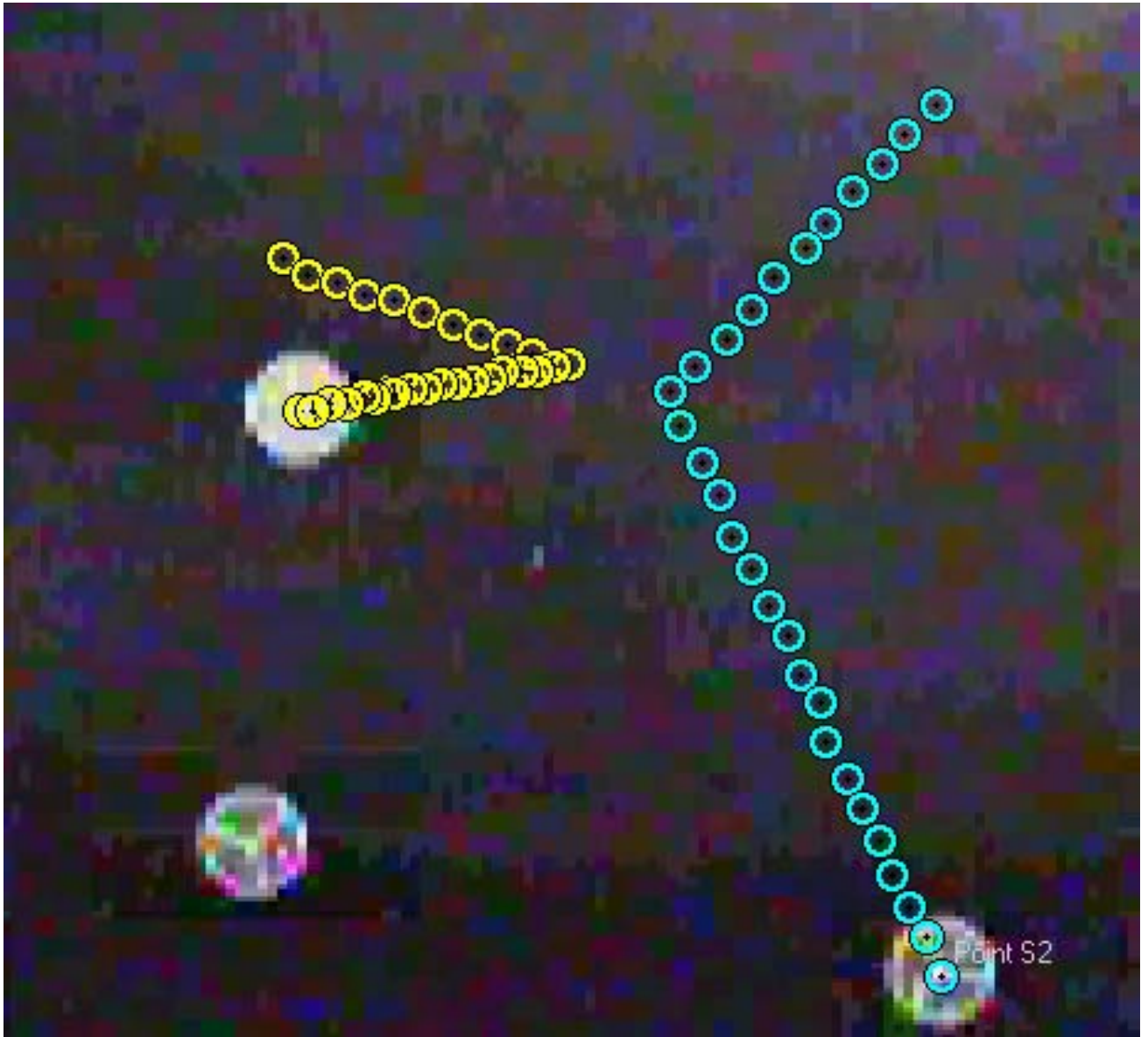
Figure for PreLab #4. This is the final frame of a video of two colliding pucks. The y -axis points toward the top of the page, and the x -axis points to the right.
