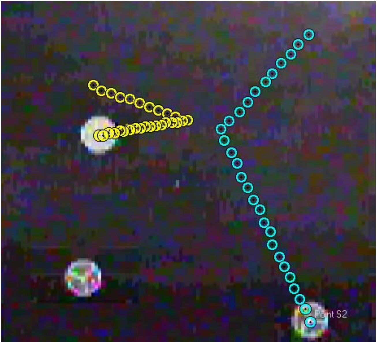
Figure for PreLab #1. This is the final frame of a video of two colliding pucks. The y -axis points toward the top of the page, and the x -axis points to the right.
