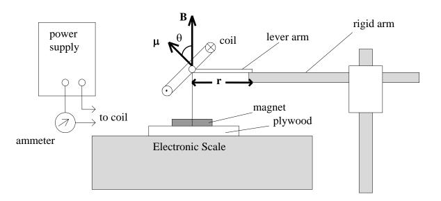
If the coil rotates away from the rigid arm when powered, reverse the leads of the motor to the power supply.
