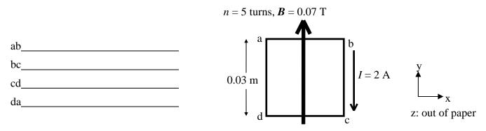
What is the magnitude and direction of the torque  $\tau$  on the coil about its center, if any? Use the fact from mechanics that  $\tau = r \times F$  due to a force F applied with lever arm r.
