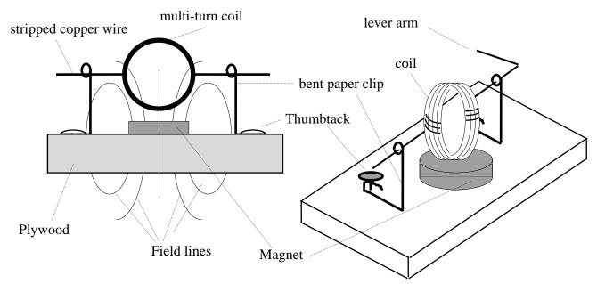
Once the motor is assembled, power it by connecting its leads to a DC power supply of about 2 volts. Always keep the voltage low enough that the current is less than 5 amps. If the coil doesn't turn, give it a little twist to get it started. If it still doesn't turn, you need to make some adjustments. Carefully bend the axles until the coil is balanced. It should rotate without too much wobbling when spun with no current applied. Check that all insulation is cleaned off the axle wire.
