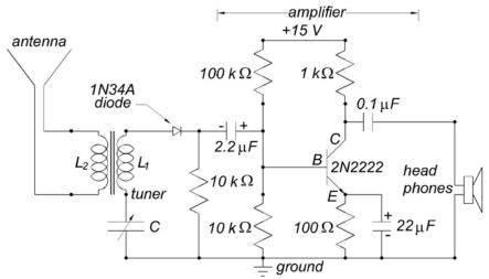
Do NOT connect the antenna to the ground of your amplifier circuit. Use the transformer!
