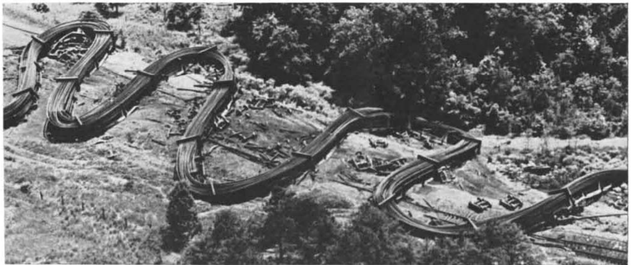
CATASTROPHIC EXAMPLE of a sine-generated curve on a much larger scale was provided by the wreck of a Southern Railway freight train near Greenville, S.C., on May 31, 1965. Thirty adjacent flatcars carried as their load 700-foot sections of track rails chained in a bundle to the car beds. The train, pulled by five locomotives, collided with a bulldozer and was derailed. The violent
