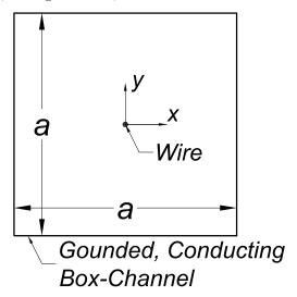
Give a series expansion the electrostatic potential V(x, y) inside the Iarocci tube supposing the wire carries charge q per unit length.
