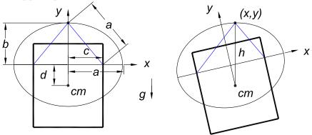
If the wire slips with respect to the support point, the latter lies on an ellipse with semimajor axis a and semiminor axis b. The center of mass of the picture still lies directly below the support point, now at distance h from it. The system is unstable against such slippage if the center of mass falls as the wire slips, i.e., if,
