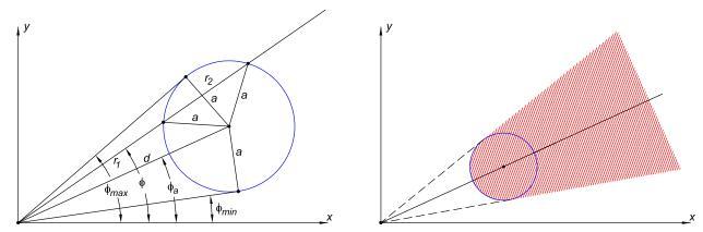
Any ray from the origin that passes through the solenoid has  $\phi_{\min} < \phi < \phi_{\max}$  where  $\phi_{\max,\min} = \phi_a \pm \sin^{-1}(a/b)$ . Such a ray intersects that solenoid at radii  $r_1$  and  $r_2$  related by,
