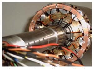
The sensors were ferrite cores with a toroidal winding, encased in an aluminum Faraday cage for electrical (but not magnetic) shielding, as shown in the photograph below. The sensors observe the azimuthal magnetic field around the axis of the ferrite cores, which is interpreted as a conduction current in the "squirrel-cage" bar that passes through the core. A sketch of the concept of an "amp-clamp" is shown on the right below, from [58].
