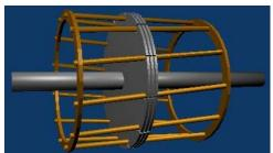
The time-dependent magnetic field of the stator induces electrical currents in the conducting loops of the "squirrel cage," such that the  $\mathbf{I} \times \mathbf{B}$  force on these currents torques the rotor, leading to rotation of the latter at almost, but not quite, that of the angular velocity of the (rotating) magnetic field of the stator.<sup>34</sup> Hence, in the rotating frame of the rotor, the magnetic field has a rather low frequency, around 1 Hz for a 50-60 Hz induction motor.
