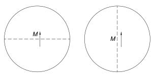
Show that the force between hemispheres in the left figure is the same as that between one such hemisphere and either a perfectly conducting plate, or a plate of infinite magnetic permeability.
