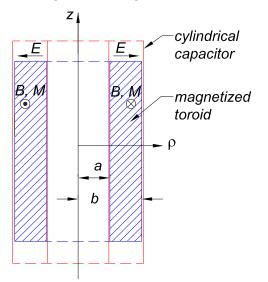
The two electrodes of the capacitor, and the toroid, can move without friction along their common axis. Ignore gravity.
