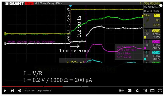
Soon after the start of the applied pulse, a small voltage (0.2 V) appeared across the load resistor, and persisted until the wave reflected off the ends of the circuit arrived at the load resistor some 1.6  $\mu$ s later. This first interval of constant load voltage is (we infer) associated
