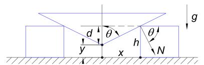
For this, we relate the vertical position y of the bottom tip of the wedge to the horizontal position x of the left edge of the right block relative to the symmetry axis x = 0, as shown
