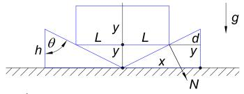
To apply Newton's  $2^{\rm nd}$  law to this problem, we note that the force of contact **N** between the wedge and the block is normal to the surface of the wedge, and hence makes angle  $\theta$  to the horizontal as shown above. The horizontal equation of motion of the right wedge is then,
