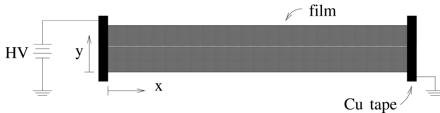
Figure 3: The application of high voltage and the set of axes used in testing the strips of carbon-loaded kapton.
