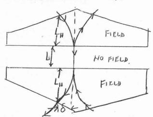
$L_{\rm H}=\sqrt{298}$  = 160 cm. Thus if L = 100 cm. The total straight section is 2 x 160  $\pm$  100 = 4.2 meters. This is not too long to be without focussing magnets in a radial sector Mark I; but since the beams are 10 cm apart, focussing with finite gradients could probably take place within the bending field even with a gap of about 10 cm width.
