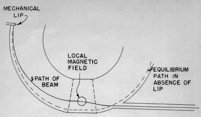
A POSSIBLE EJECTION MECHANISM TO TRANSFER BEAM TO TUBE LEADING TO STORAGE RING.
