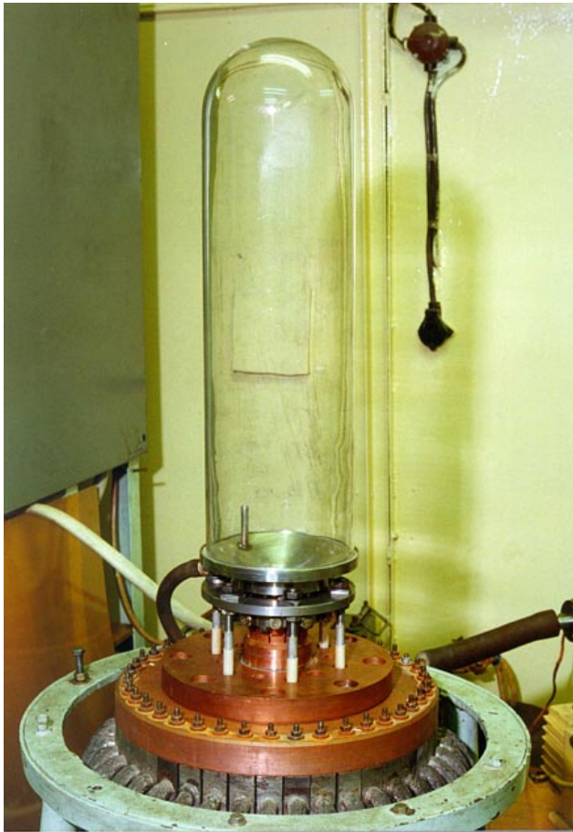
Fig.23. Photo of a device for investigation of a electromagnetic methods of liquid metal acceleration.
