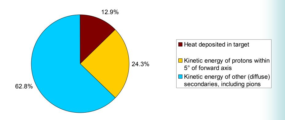
Figures from a **10GeV** proton beam (ISS baseline) hitting a 20cm long, 2cm diameter tantalum rod target
