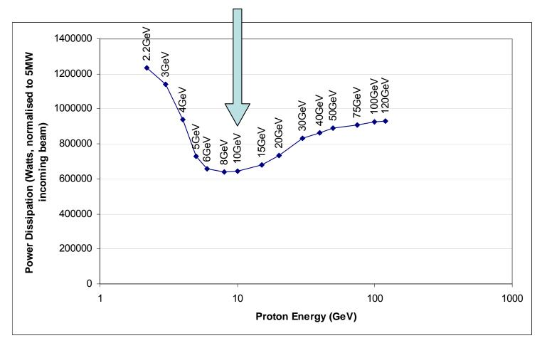
Scaled for 5MW total beam power
