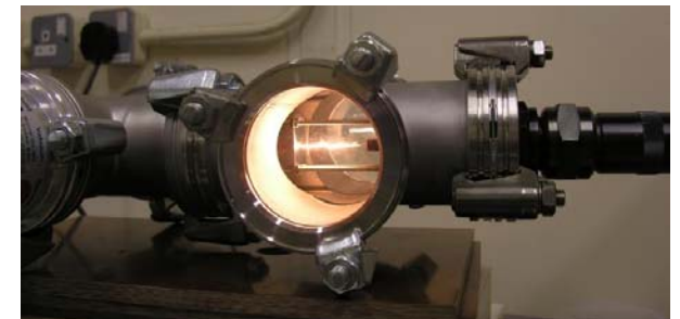
lifetime testing of tungsten wires in response to dynamic thermal loading, Skoro et al.
