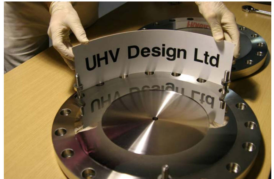
Polished flange (surface roughness, R_a = 0.020 \mu\text{m} )
