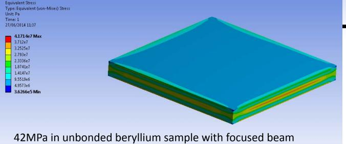
Maximum temperature and stress in samples depends on beam size, sample shape, and attachment to cooled back plate.
