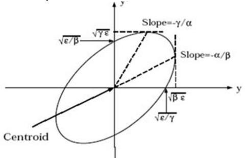
2. 2-D Transverse Emittance (rms) and Twiss Parameters
