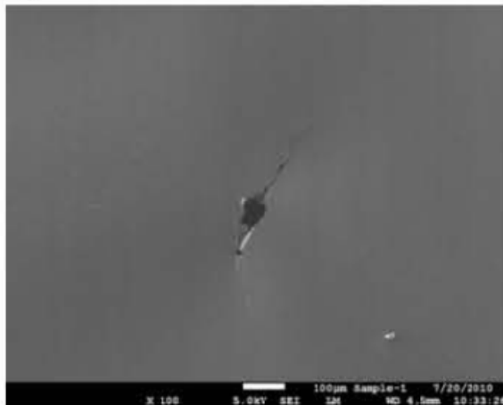
SEM photographs of unused carbon foil (left) showing a small pinhole for illustration and a foil exposed to 8.1 MeV/u Pb beam
