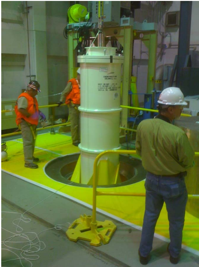
PBW Cask Liner is Loaded into the Service Bay
