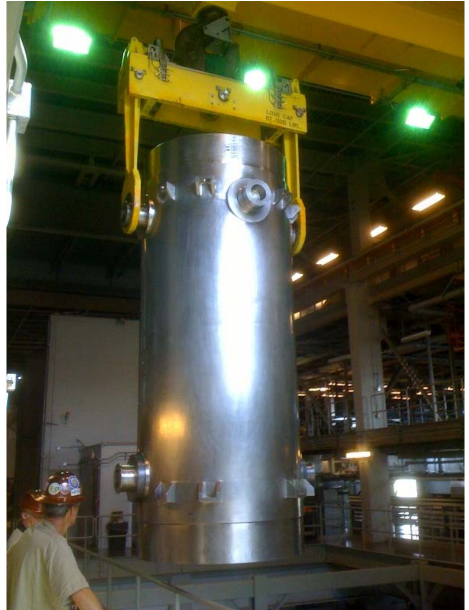
Translating Cask over for Lowering into Cask Cart
