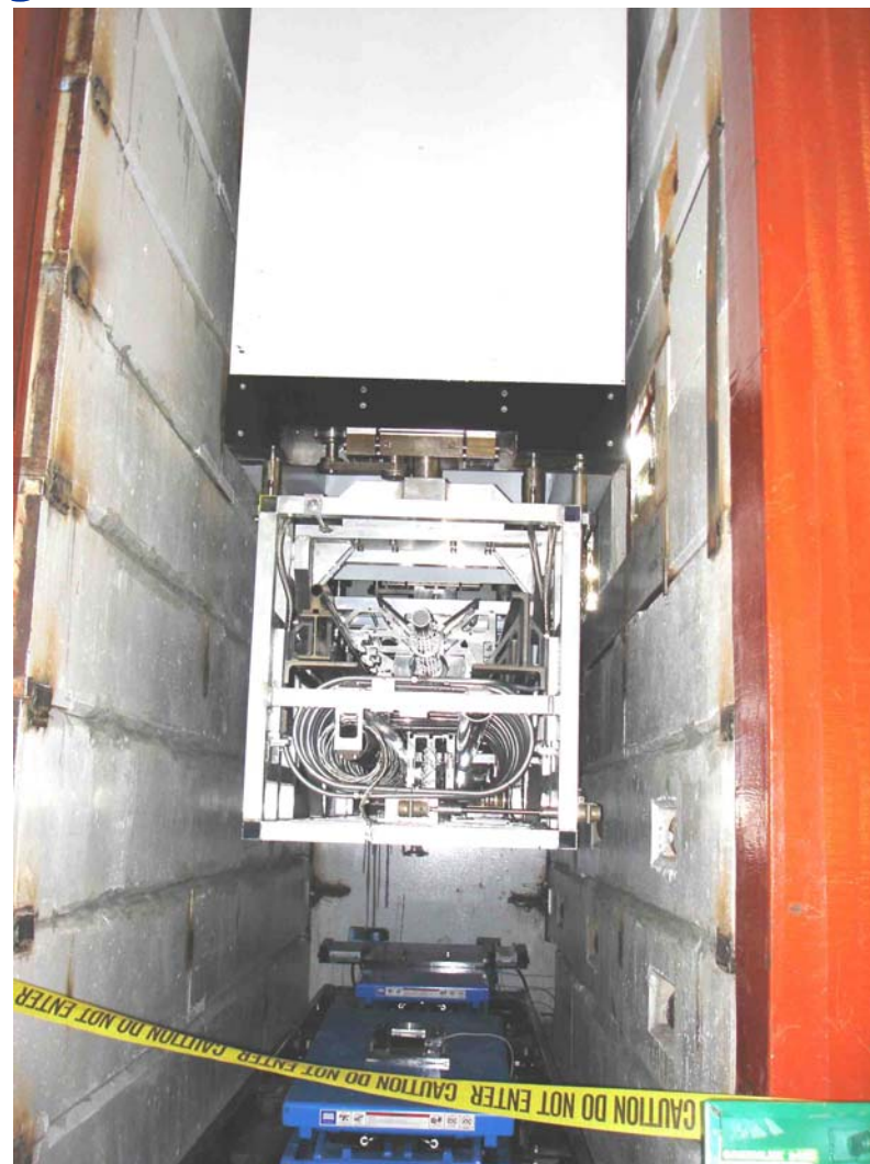
Target on module, ready to crane into beam
