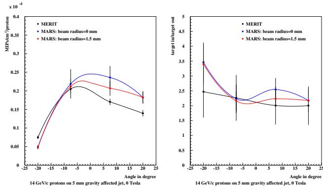
Fig. 9. Left: The response of the pCVD diamond detectors installed at different angles around the mercury target for a 14 GeV/c proton beam compared to MARS simulation predictions. Right: The ratio of the response with and without the mercury jet for experimental data and simulations. The MARS simulation was done for a pencil like proton beam and for a beam with radius of 1.5 mm.
