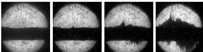
Fig. 6. A 1-cm diameter, 15-m/s Hg jet at 0, 75, 175, and  $375 \mu\text{s}$  after interaction with  $10 \times 10^{12}$  24-GeV protons in a 10-T solenoid field.
