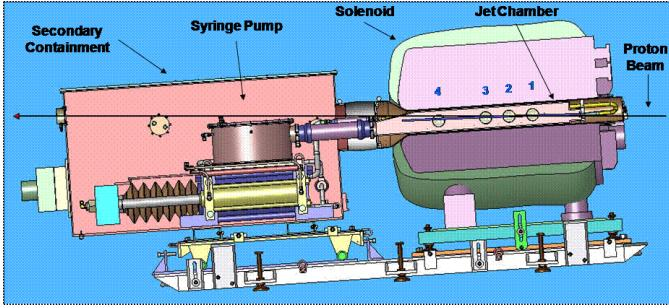
Fig. 2. Schematic view of the experimental apparatus. The mercury delivery system with its sump and syringe pump is shown on the left. On the right is the solenoid with the special primary titanium container inserted from the downstream part.
