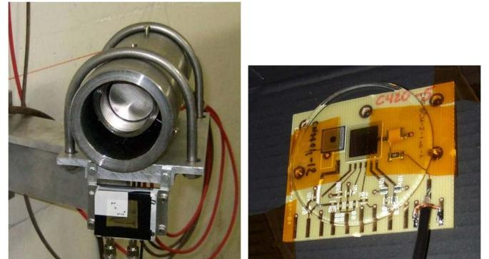
Fig. 4. Left: photo showing one detector assembly: the ACEM detector is located at the top with the pCVD diamond box at the bottom. Right: the board housing the pCVD diamond detector (center) and a pin diode (top left).
