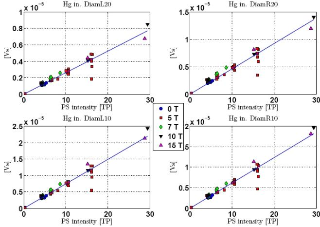
Fig. 8. The response linearity of the pCVD diamond detectors for increased beam intensity.(1 TP corresponds to  $10^{12}$  protons on target).
