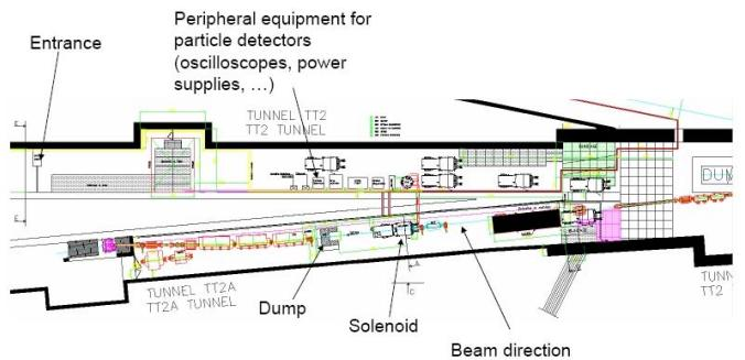
Fig. 1. The experimental setup in the TT2/TT2A tunnels of CERN PS. The beam arrives from the right side of the figure and after traversing the experiment is stopped in an iron dump before reaching the nTOF target shown on the left.
