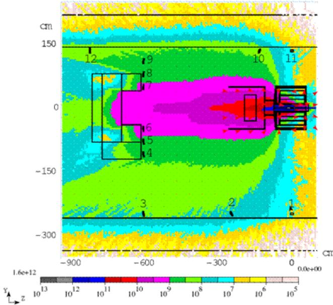
Fig. 5. MARS simulation showing the charged hadron flux per square centimeter for an incident proton beam of 24 GeV with  $30 \times 10^{12}$  protons on the MERIT target and with the solenoid field at 15 T. The location of the particle detectors around the experimental setup is shown.
