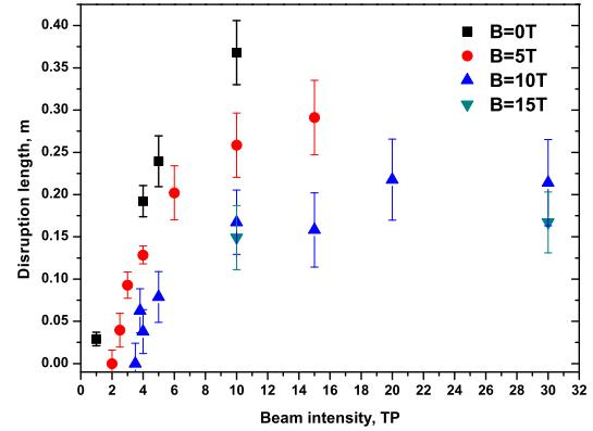
Fig. 7. The observed disruption length of the Hg jet for various beam intensities and solenoid field strengths for an incoming proton beam energy of 24 GeV.
