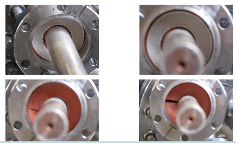
Taking out the G10 and looking at the first (left) and second (right) rubber ring
