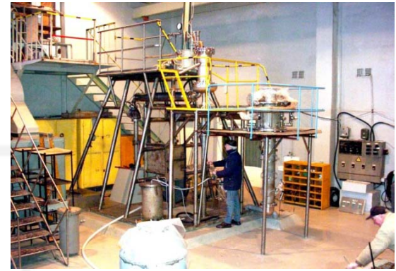
Existing Hg – loop in Institute of Physics) parameters of EMP p=4 bars; Q~12l/s
