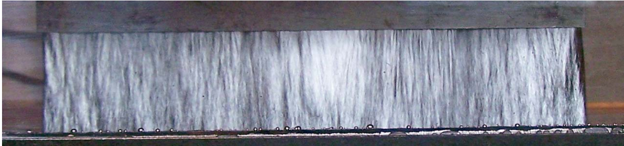
Section 3 with ~300mm long and 16 mm width. Flow velocity of 2.2 m/s
