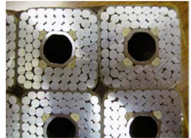
The stranded conductors impregnated by the polyimide resin to form the coil
