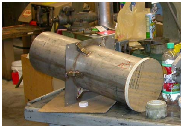
Roof penetration finally welded – waiting for warm weather for installation !
