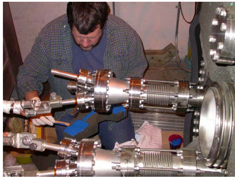
Dave Tracey Bonding Insulation with Stycast to MERIT Pulsed Magnet Cover
