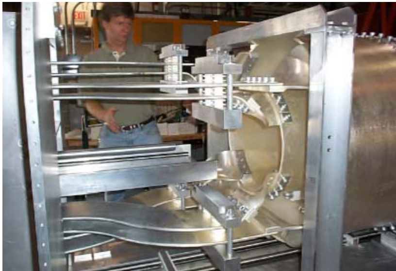
Stripline plates with smooth transitions
