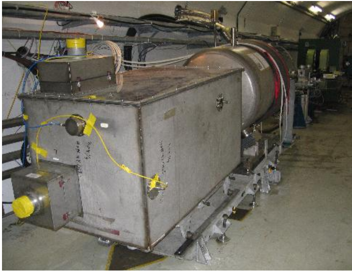
Magnet mated with the Hg injection system: Pulsed High-Field Solenoid
