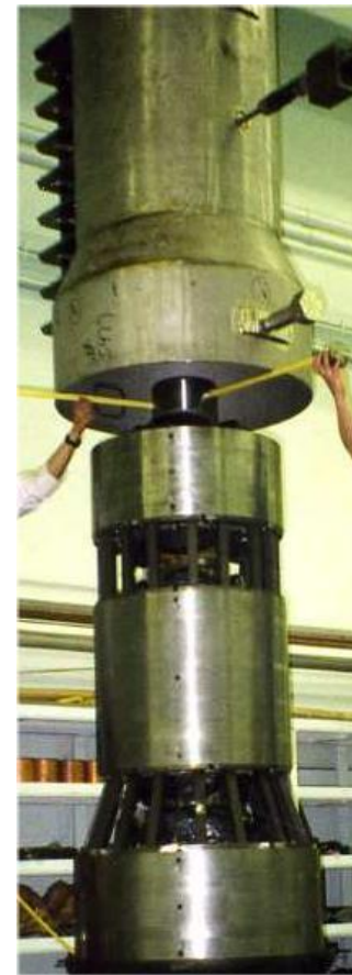
Inserting the cold assembly into the helium vessel
