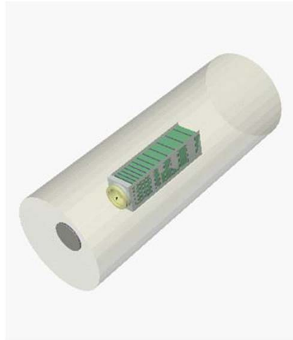
Figure 1 Simplified ISIS geometry used for FLUKA model
