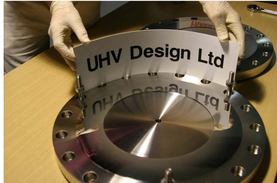
Polished flange (surface roughness, R_a = 0.020 \mu\text{m} )
