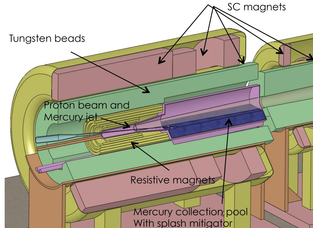
5-T copper magnet insert; 10-T Nb<sub>3</sub>Sn coil + 5-T NbTi outsert.
