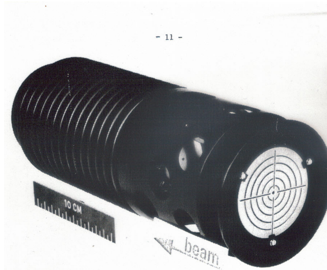
Fig. 5 - Overall view of the target assembly. The aluminium container is anodised black to aid cooling via radiation. The hole in the upstream luminescent screen avoids premature aging and radiation damage of the latter.
