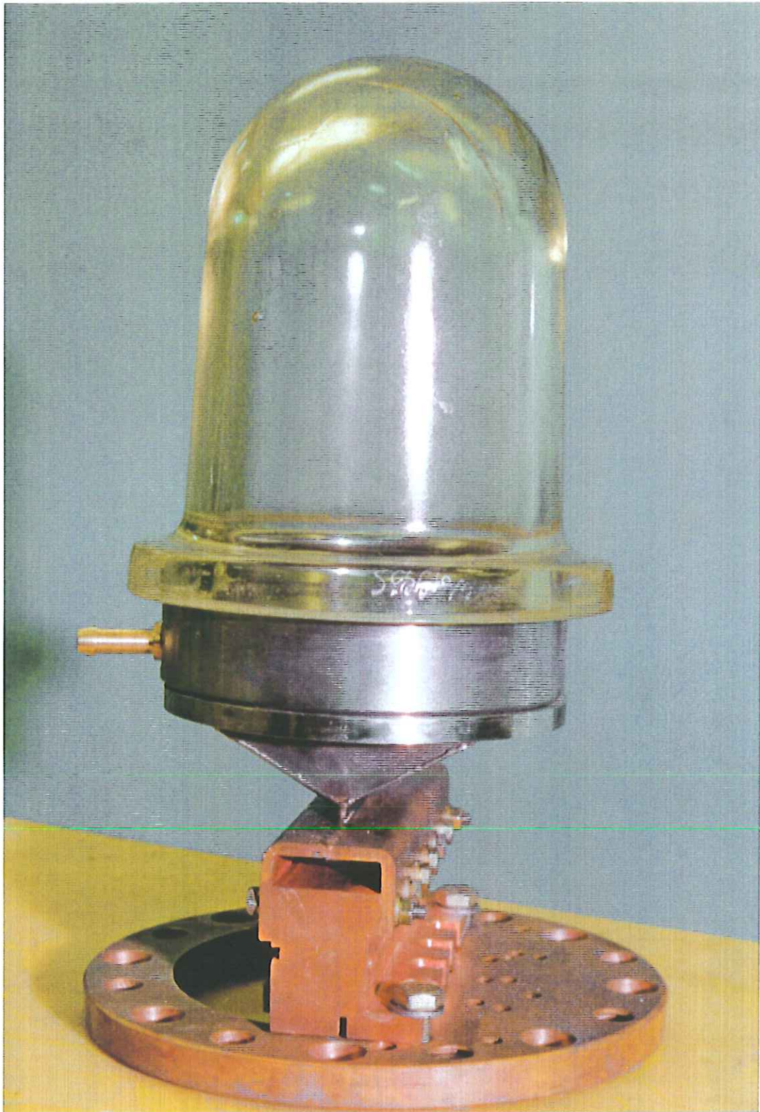
Fig.15. Photo of a target device prototype for vertical flat jet formation.
