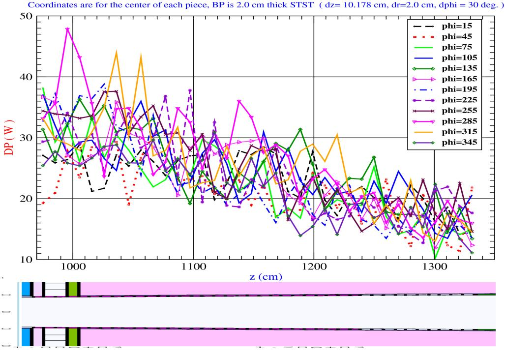
DP vs. z for BP#2 from 970.0 < z < 1336.4 cm (~ CRYO#3), for 12 angles
