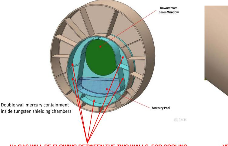
He GAS WILL BE FLOWING BETWEEN THE TWO WALLS FOR COOLING. THE BEAM PIPE IN THAT AREA WILL BE PART OF THE POOL VESSEL AND REMOVING THE HEAT LOAD WILL BE A CHALLENGING TASK. SEGMENTATION ANALYSIS WILL BE PERFORMED TO DETERMINE THE AZIMUTHAL DPD DISTRIBUTION.
