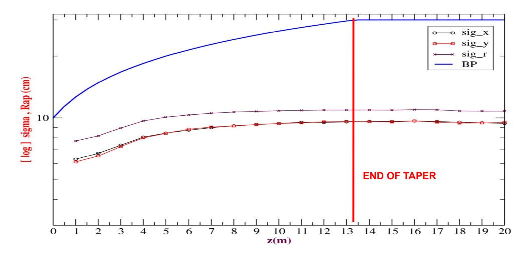
x AND y SPREADING HAVE ONLY A SMALL DIFERENCE. FROM THE RADIAL SPREADING WITHIN THE FIRST 10 m OR SO IT APPEARS A PORTION OF THE PARTICLES COULD BE LOST IN THE BEAM PIPE AND SHIELDING MATERIAL. THE RADIAL SPREADING HAS REACH ITS LIMIT VALUE OF ~ 11 cm AT z ~ 10 cm. [GAUSSIAN DISTRIBUTION ?]
