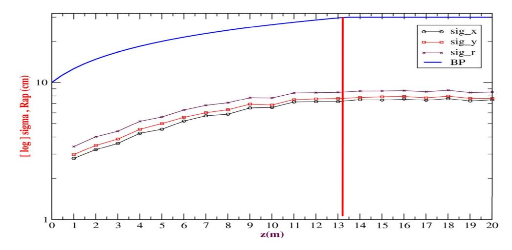
x AND y SPREADING IS MORE ASYMETRIC THAN THAT OF PIONS. RADIAL SPREADING LIMIT IS ~ 9 cm AND THERE IS A COUPLE OF METERS REGION (7-9 m) WHERE A RELATIVELY SIGNIFICANT NUMBER OF MUONS COULD BE LOST IN THE SHIELDING.
