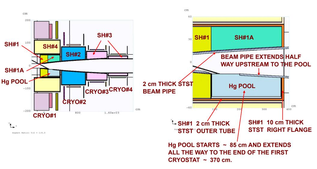
SHVS WALLS, Hg POOL VESSEL DOUBLE WALLS, Be WINDOW, He GAP IN BE WINDOW AND IN HG POOL HAVE NOMINAL VALUES FOR THEIR THIKNESS. STRESS FORCES ANALYSIS AND LOCAL DPD DISTRIBUTION WILL BE USED TO DETERMINE THEIR VALUES.
