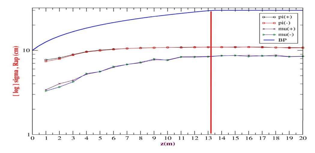
MUONS RADIAL SPREADING HAS A FASTER INCREASE WITHIN FIRST FEW METERS SINCE MORE AND MORE PIONS DECAY TO MUONS INCREASING THEIR NUMBER AND THEIR SPREADING.
