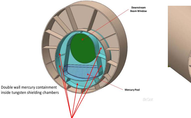
He GAS WILL BE FLOWING BETWEEN THE TWO WALLS FOR COOLING. THE BEAM PIPE IN THAT AREA WILL BE PART OF THE POOL VESSEL SHIELDING. REMOVING THE HEAT LOAD WILL BE A CHALLENGING TASK. SEGMENTATION ANALYSIS WILL BE PERFORMED TO DETERMINE THE AZIMUTHAL DPD DISTRIBUTION. VESSEL FILLED WITH He CO W BEADS FOR SCs
