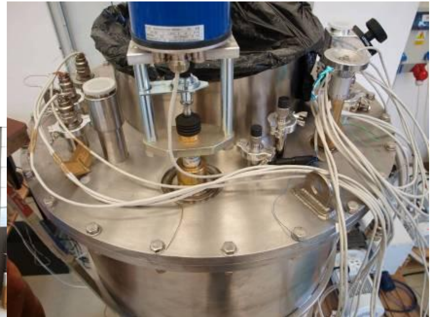
Top view of the cryostat with wiring
