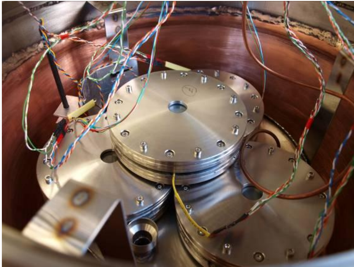
4 sample holders in the measurement vessel
