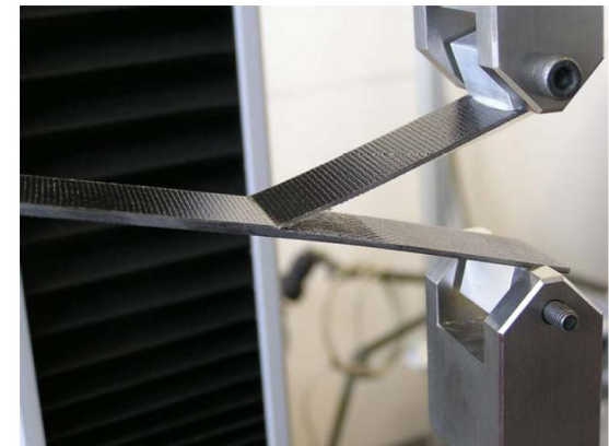
Interlaminar fracture toughness test
