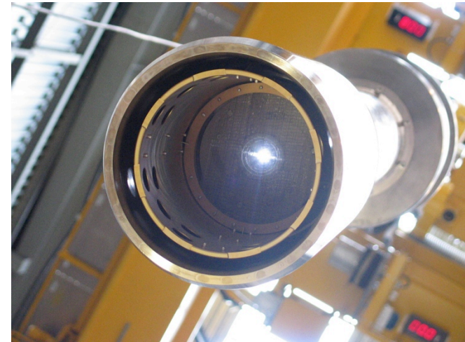
VIMOS insert with Tungsten mesh
