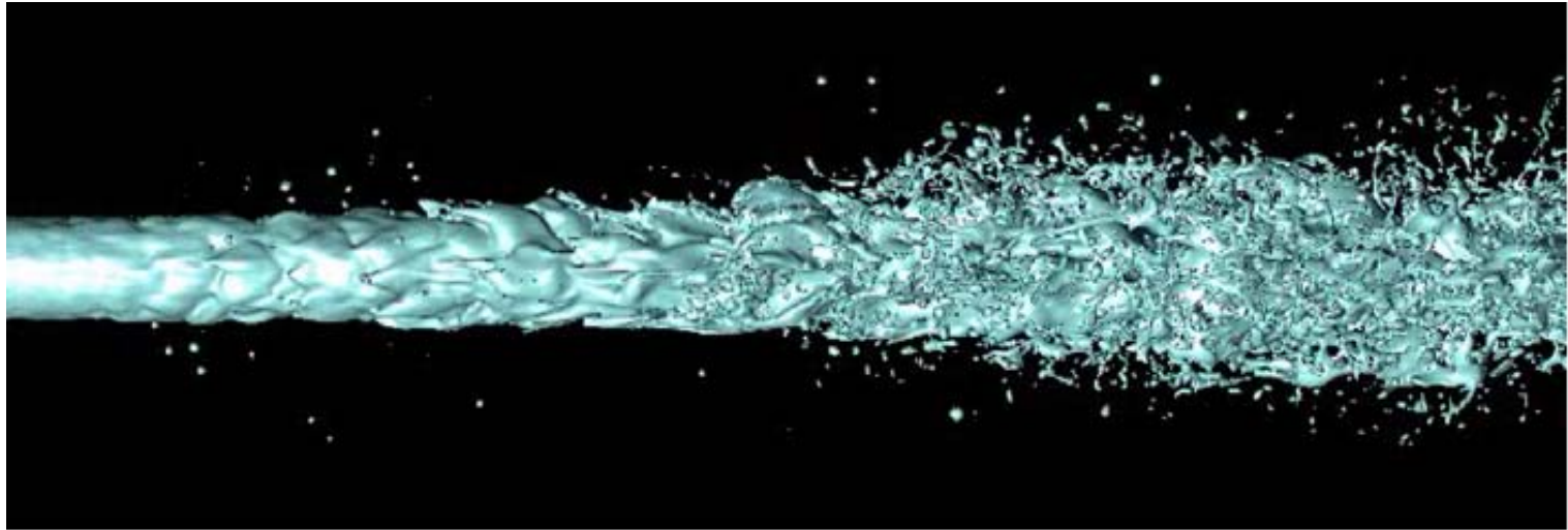
Fig. 11 (b) Liquid jet surface and break-up near the jet nozzle
