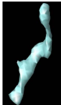
Fig. 11 (b) Liquid jet surface and break-up near the jet nozzle
